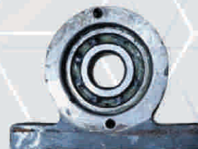
CSP/8: [Axle Bearing & Cover (6206 RS)]
